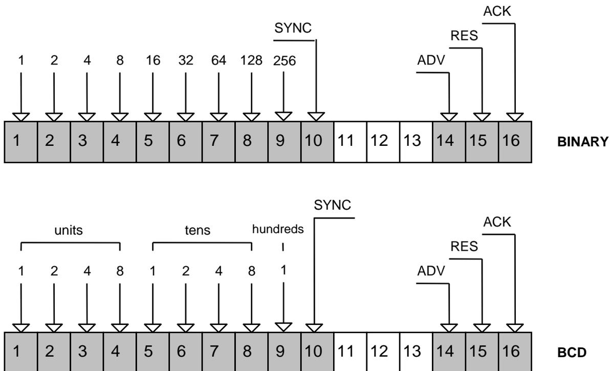
In this operation mode, three function inputs are available, in addition to the message recall inputs (ADDRESS + SYNC):
