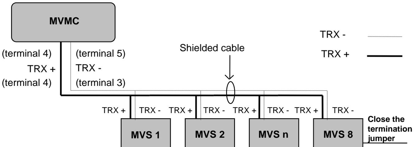
**NOTE 1.** The RS485 connection is multidrop; therefore the bus termination resistance must be selected on the last card of the connected multiplexer, by closing the removable jumper; this jumper must be open on the intermediate multiplexer cards.
