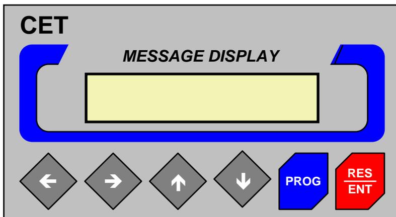
**→← CURSORS** for horizontal right or left movement, used to move inside the programming menus; in code programming they move the cursor.
