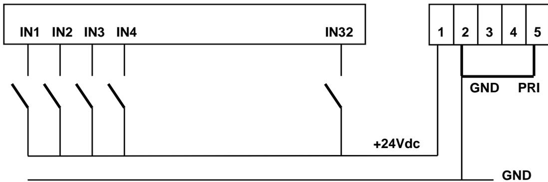
Note: the programming of the Contact Logics ACTIVE CLOSED or ACTIVE OPEN, carried out by means of the dip 2 from the MVMC menu or using the WINTEXT programming software, does not depend on the Positive or Negative Logics connection.
