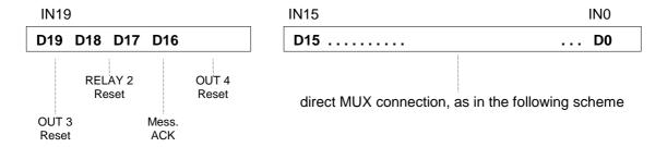
Complete connection diagram between A402 and MUX64/A
