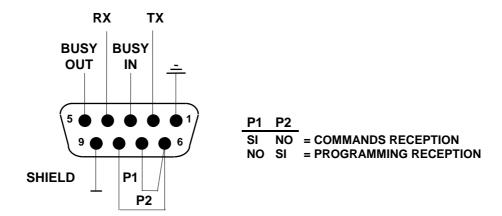
The two P1 and P2 bridges determine the type of connection and therefore the operations to be carried out. With the serial line it is possible to carry out the following functions:
