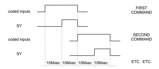
The input signals, managed with MUX64, answer with times from MUX; in general the total scanning time of the 64 input CONTACTS is (:)93 Sec., whether, there is only one input or they are all connected.
