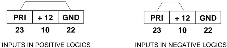
The terminal board supplies an outside power supply of 12VDC (100mA) which can be used to control the inputs as an alternative to the external power supply, according to the following scheme (only for inputs programmed in positive logics).
